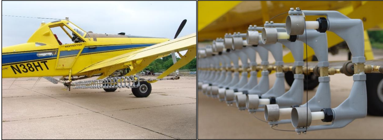
Figure 2. (a) USDA-ARS Air Tractor 402b used in the 2017 Texas pilot project and (b) a close-up view of the nozzles.
