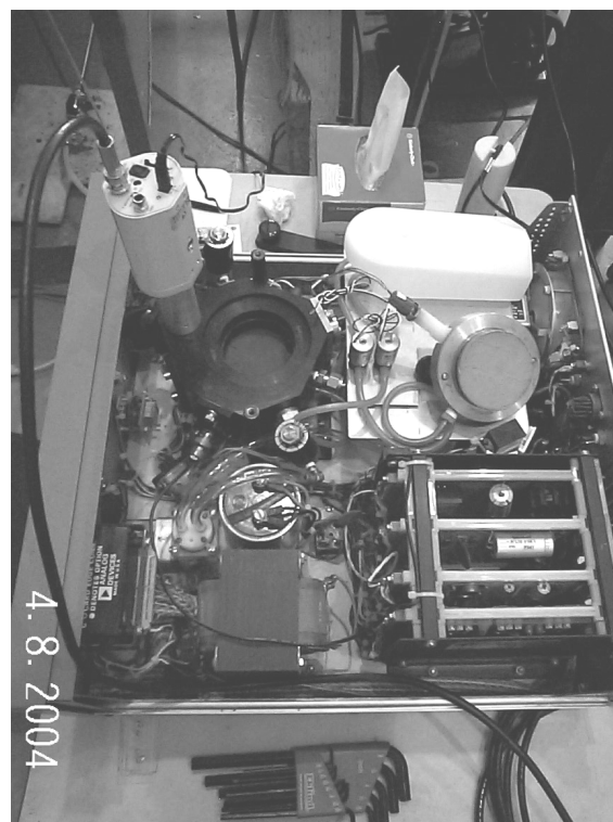
Figure 1: A view, looking down on the open case of the SDSMT Mee CCN counter. The cloud chamber is open, with the upper plate lying to the right, and the base of the chamber in the center left portion of the image. The blotter-paper-covered inner plate surfaces are 10 cm in diameter, and the spacing between the plates, when the chamber is assembled, is 1 cm. The video camera in the upper left of the picture looks into a mirror set at a 45° angle to allow a view of the inner chamber. The white plastic bottle in the upper right of the image is the water reservoir for the system used to keep the inner plate surfaces moist.
