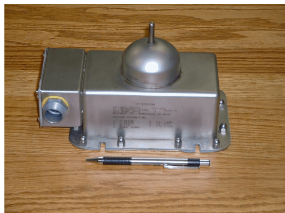
Figure 2. Rosemount ice detector, model 872B.
