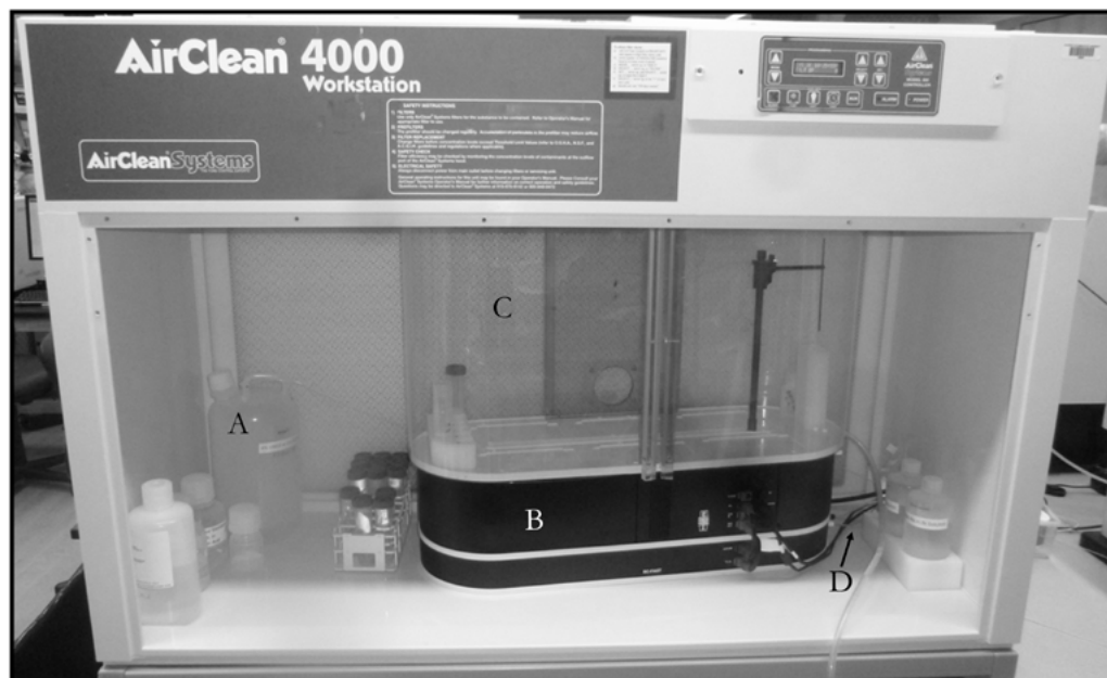
Figure 3: A) 4% \text{HNO}_3 rinse solution B) Autosampler C) Plastic cover surrounding the autosampler D) Tubing delivering sample from the autosampler to the ICP-MS.
