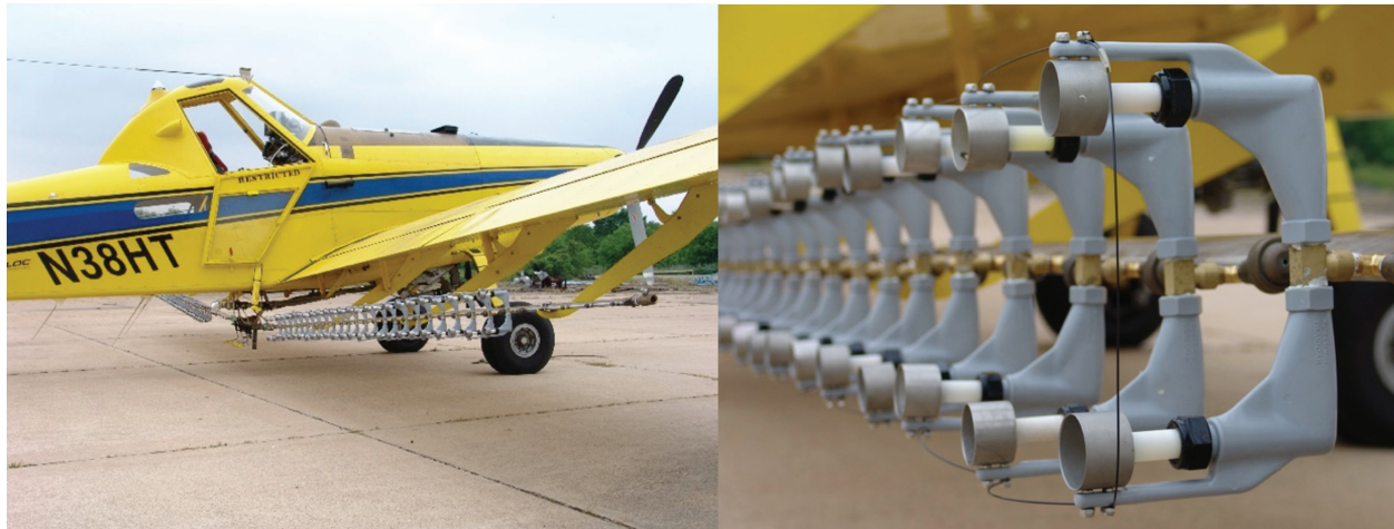
Fig. 2. (Right) USDA-ARS Air Tractor 402b used in the 2017 Texas pilot project and (left) a close-up view of the nozzles.
